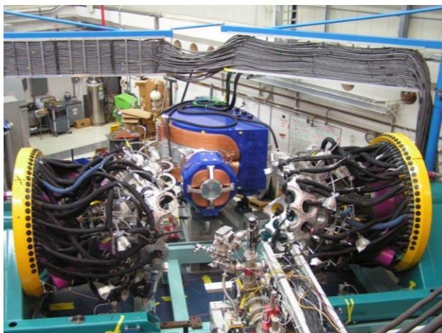
The GAMMASPHERE germanium detector array located at the focal plane of the newly commissioned AGFA gas-filled spectrometer.
