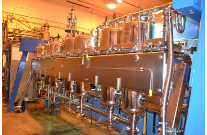
A string of superconducting cavities and focusing solenoids developed for a recent intensity upgrade of the ATLAS facility.
