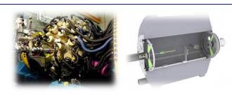
GAMMASPHERE, an array of over 100 Comptonsuppressed Ge detectors, and HELIOS, a novel superconducting solenoid spectrometer, are examples of forefront instruments which are available for experiments at ATLAS.
